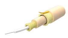
Fiber indoor/outdoor drop cable, All-Dielectric, 1 fiber Tight Buffer construction, riser, drop all-dielectric, Singlemode G.657.A2, Gel-free, Feet jacket marking, Ivory jacket color
