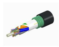
Fiber OSP cable, LightScope ZWP® Single Jacket/Single Armor, 96 fiber, Gel-Free, Stranded Loose Tube, Singlemode G.652.D and G.657.A1, Meters jacket marking, Black jacket color
